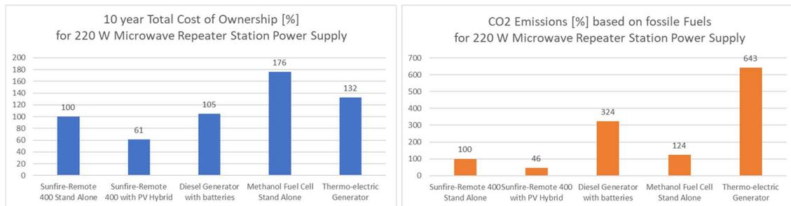
Fig. 2: Comparison of 10-year TCO and CO<sub>2</sub>-Emissions of the different Solutions
